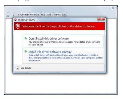
The installation will now finish, close the window and turn off the signal generator. Turn the signal generator on and start the Torchmate driver program. Select 'Yes, Start Online" and the software will communicate with the signal generator.
