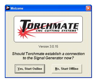
To ensure that the signal generator's drivers were installed properly have the signal generator on and select 'Yes, Start Online'. The Torchmate driver software will attempt to establish a connection with the signal generator.
